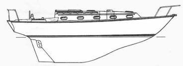
The Cape Dory 33 is a masthead sloop with powerful lines and is easily driven, responsive and stable. Like every Cape Dory yacht, the Cape Dory 33 has the Alberg-designed full keel and attached rudder.
