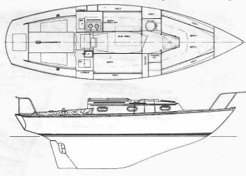
The Cape Dory 27 is a diesel powered auxiliary sloop capable of sailing most anywhere. She is a rugged, Alberg-designed yacht, with surprising speed and predictable handling of a full keel design. The 27 is an uncomplicated yacht universally admired by knowledgeable sailors. She's an ideal cruiser with standing headroom, a complete aft galley, and berths for four. Privacy is provided
