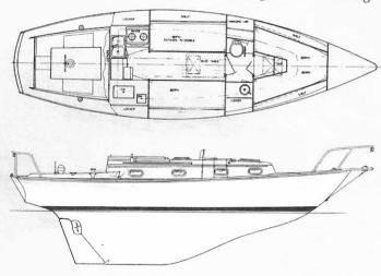
The Cape Dory 30 was designed by Carl Alberg to meet the needs of the serious cruiser. There are berths for five, including a double, in the two cabins. The head is accessible behind closed doors from either cabin, and there is ample locker and storage space throughout the cabin. The galley has been designed to include generous storage areas and efficient use of space. A gimballed stove with oven is standard, as is the large, fully-insulated, top-loading ice box.
