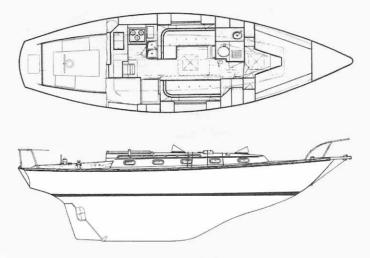
The Cape Dory 36 is a true blue water cruiser, yet she is equally well suited for the gentle breezes of an afternoon sail. Carl Alberg designed the 36. She features a "full keel" with attached rudder and a cutter rig - important features which assure stability and short-handed sailing ease.
