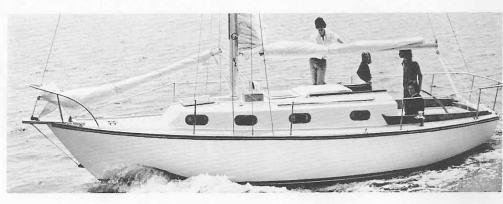
Mr. Alberg then in his design insured an ease of handling and a boat with a good turn of speed. We felt that one or two people should be able to comfortably sail the 28 with a minimum of sail handling so we included as standard a self-tending jib boom and jiffy reefing on the mainsail.
