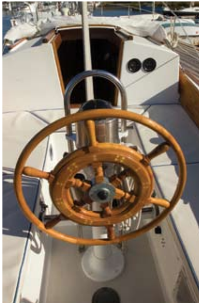
Pedestal steering makes Good News IV unusual among Cape Dory 27s, creating additional room for passengers in a cockpit considered spacious in its day.
