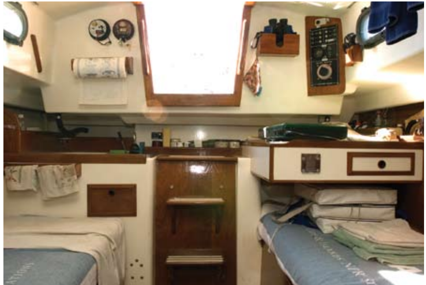
When looking aft in the main cabin, the galley sink is to the left and the cooking space is to the right. Access to the diesel engine is gained by removing the wooden panel and companionway steps in the center of this photograph.
