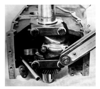
**68.** Fit the governor. Tighten it in position with the set screw on the side. See that it goes into the groove.
