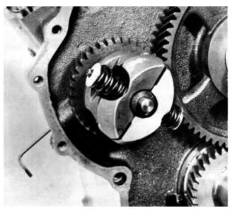
**69.** Fit the gearwheel on the camshaft's opposite end.
