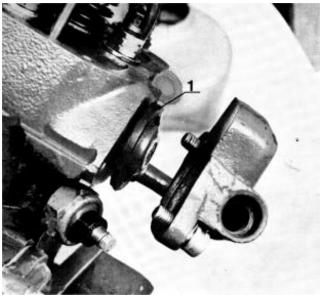
**85.** Place the key for the gearbox connecting drive on the crankshaft on the gearbox side. Heat the connecting drive and fit it onto the crankshaft. Lock the drive with the large washer and the lockwasher. Tighten the screw with a torque wrench. The tightening torque is 70 Nm (7 kpm) (50Lbft.). Use a counter force. Bend the lockwasher up against the screw head afterwards.
