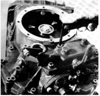
centre screw on the tool until the flywheel loosens.
