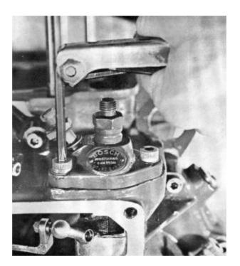
screw (1), the governor and the gear wheel can then be withdrawn.
