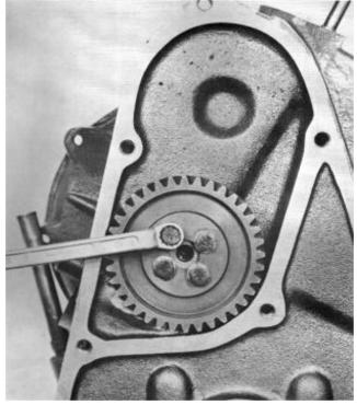
**14.** Remove the cover (flywheel side), 10 screws. The cover is centred with guide pins. The screws by the guide pins are fitted with thick washers.
