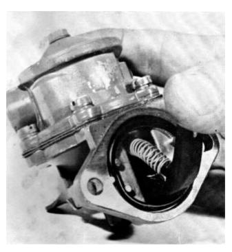
$\ensuremath{\textbf{29.}}$  Remove the cover's centre screw, remove the filter 1 and clean it.
