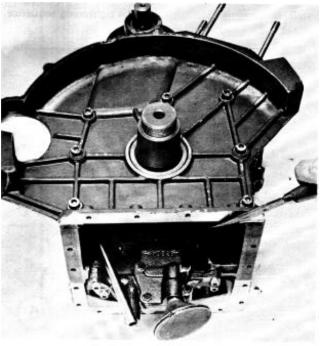
**77.** Fit a plane packing and then fit the sump. Note! On earlier engines a rubber seal was used. This is to be replaced by a plane packing.
