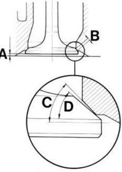
**50.** Adjust the length of sleeve protruding from the cylinder head face, (length is 0,9 mm) (0,0354 in.) and check that the sleeve is correctly fitted (dimension 19,5 mm). (0,7677 in.).
