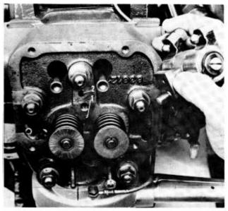
**78.** Lubricate and replace the valve lifters. Fit a new cylinder head gasket and then the cylinder head. Place the washers under the nuts and tighten the nuts in three stages to 70 Nm (7 kpm) (50Lbft.). See the tightening sequence. First stage: 10 Nm (1 kpm) (7Lbft.). Second stage: 40 Nm (4 kpm) (29Lbft.). Third stage: 70 Nm (7 kpm) (50Lbft.).
