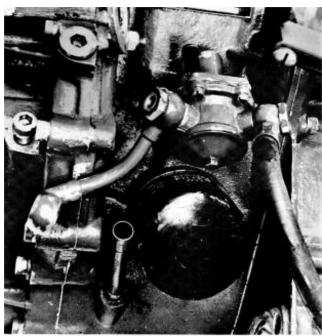
**81.** Fit the fuel filter. Place sealing rings on both sides of the fuel pipe unions.
