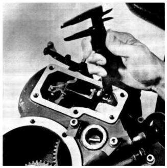
**73.** Release the plunger 8 mm (0,3150 in.) and measure the distance from the transmission cover face to the adjusting screw's contact point on the control arm.
