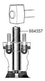
**49.** Lubricate the mandrel tool 884537 and insert the tool into the sleeve. (Ensure that the centre screw is sufficiently unscrewed.) Place some nuts or several washers on the studs so that the yoke can be tightened in place with the fixing nuts. Screw in the mandrel as far as the mating face of the sleeve allows. The mandrel is then withdrawn. Remove the tool.
