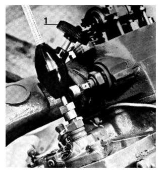
**92.** If the injection angle does not meet the prescribed value, the number of washers 1 between the pump housing and the transmission cover is increased or decreased until the correct value is obtained. One washer gives a difference in injection angle of approximately 1°.
