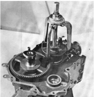
**13.** Remove the lubricating oil pump. Discard the gasket.
