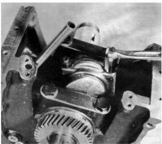
**17.** Remove the main bearing caps. Take care of the axial thrust bearings 1 on the transmission side. Lift the crankshaft out and the bearing shells afterwards and then the axial bearing halves.
