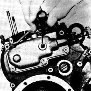
**74.** Measure the adjusting screw's length and adjust any eventual deviation so that the plunger stops when released 8 mm. Screw down the cover afterwards.
