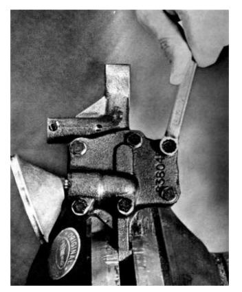
**22.** Remove the gearwheel from the housing. Remove the split pin for the reduction valve. Remove washer 1, spring 2 and piston 3. Clean and replace damaged parts. Assemble the lubricating oil pump in the reverse order. Note! Fit a new gasket 4 between the housing and the cover. Fix the wire mesh 5 in position with the steel wire 6 and finally lay the key in position and tighten the gearwheel 7.
