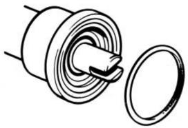
**24.** Remove the cover (6 screws). Change the impeller with the help of two screwdrivers or something similar. Note! Protect the edges of the pump housing. See the figure. Prise out the impeller with the screwdrivers so far that the screw becomes visible.
