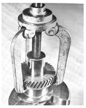
**36.** Place the key in the crankshaft's key slot. Heat the gearwheel to approximately  $100^{\circ}C$  ( $212^{\circ}F$ ) (no more) and press it onto the crankshaft. Note! The marking on the gearwheel shall face outwards. Refit the circlip on the crankshaft.
