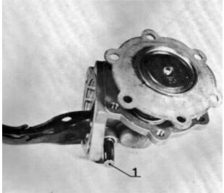
**30**. Remove the six screws which hold the upper and lower pump halves together. Remove the pump's spring and undo screw 2 which holds the pump arm spindle.
