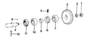
**58.** Replace damaged parts and reassemble the pin, seal, ball bearing and spacer ring on the shaft. Fit the spacer washer into the cover and tighten it in position with the set screw. Note! Ensure that the spacer washer's groove faces the locking screw's centre. Fit the shaft in the cover. Place the key in position and then the ball bearing. Fit the gearwheel. Secure it with a washer and nut. Knock out seal 1 from the flywheel cover. Press in a new seal afterwards.
