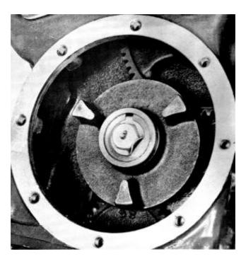
**86.** Place the key for the flywheel in the crankshaft's key slot. Fit and tighten the flywheel. Use a counter force in the spokes of the flywheel. The tightening torque is 500 Nm (50 kpm) (362Lbft.). Spanner jaw width is 55 mm (2 5/32").
