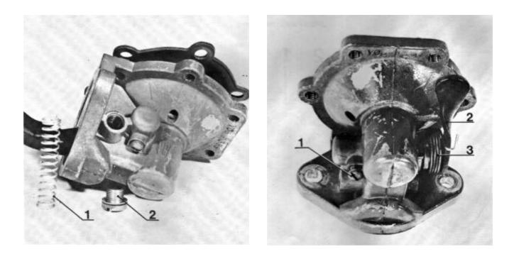
**33.** Clean the pump housing carefully and replace worn parts. Refit the manual pump arm. Press in the diaphragm and connect the pump arm to the diaphragm centre pin. Then push the spindle in and tighten it with the screw. Note! Do not forget the washer under the screw.
