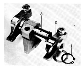
**53.** Check the wear on the rocker shaft. Also check that the tappet adjustment screw's spherical part is neither deformed nor worn. The threads on the screw and the locknut must be undamaged.
