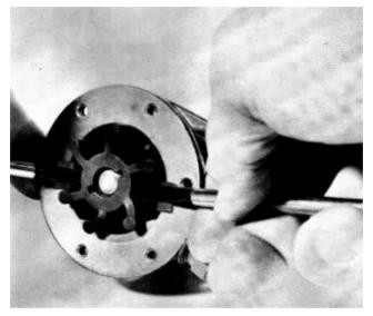
**25.** Unscrew the screw and withdraw the impeller from the shaft. If the sealing rings are to be replaced, the shaft and the impeller can be removed and the screw subsequently loosened.
