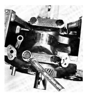
**19.** Bearing replacement. Press out the camshaft bearings if they are damaged or if the wear is too great (see technical data). Clean the bearing housings and ensure that the oil channels are clean. Press in the new bearings so that the oil holes face the corresponding oil channels in the block. When the bearings are pressed in position they are to be reamed (see technical data).
