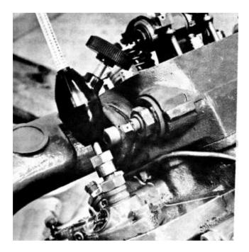
**90.** Rotate the engine in the correct direction until the level tube 1 is full with air-free fuel.
