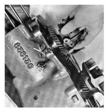
**10.** Remove the sump and then the transmission cover (13 screws). The lifting eye is fixed one of the screws. The cover is centralised by guide pins.
