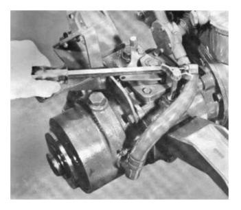
**3.** Remove the rocker cover and the fuel pipe between the pump and the injector and unscrew the rocker gear. Note! Pull the rocker gear straight up since it is centred with a guide pin 1. The other hole 2 is an oil channel.
