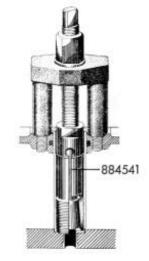
**46.** New valve guides are fitted with tool 884549. Use a press. This tool gives the guide the right height above the cylinder head's valve spring seat surface. Check the dimension "A" - this must be 9 mm (0,3543 in.) when the guide is pressed into place.
