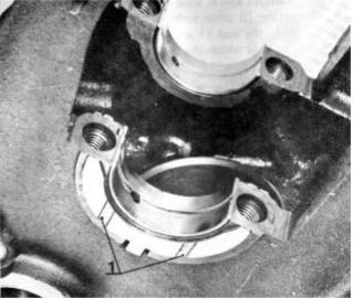
**62.** When the cylinder liner is fitted in the block the height of the liner outside the block must be measured. The height must not exceed 0,05 mm (0,0020 in.) and must not be less than 0,01 mm (0,0004 in.), otherwise there is a risk that a leak can occur.
