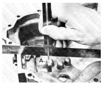
**60.** If the transmission cover is damaged and must be replaced, this means that even the camshaft and the camshaft gear must be replaced. The replacement is necessary because the axial guide in the new transmission cover is shortened by 3 mm (0,1181 in.) which in turn means that the camshaft will have an axial play of 3 mm (0,1181 in.).
